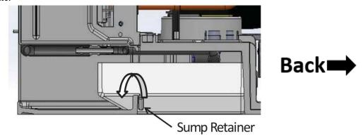
2. Once the support tabs are fully removed from the frame, let the back of sump fall downward.
