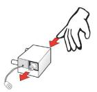
5. Pull the remainder of the bulb from the "pin-end". Remove either end cap from the bulb if it remained attached.
