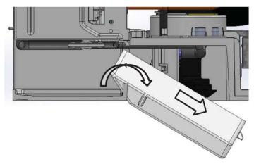
4. To re-install, reverse steps 1 through 3 and tuck the water pump tube into the sump after the sump is in place.
