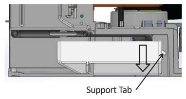
3. Similar to step 1, lift the front of the sump and push backward to allow the retaining features on the sump to clear the frame. Push down towards the back until the sump is free from the frame. Turn the sump sideways and remove it through the ice drop zone.
